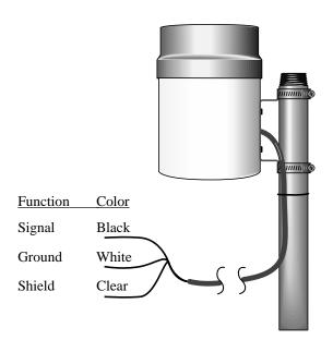
FIGURE 1. TE525 Tipping Bucket Rain Gage
